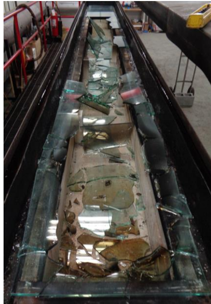
Photo No. 3 Unexposed Surface of the Test Specimen (Post-test)
