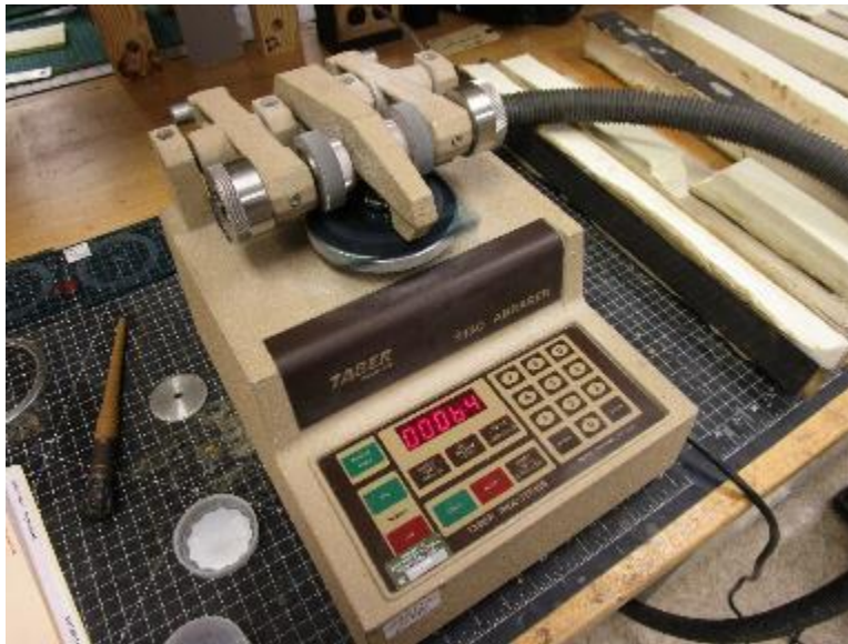
Photo No. 1 ASTM D1044 Abrasion Resistance Test Setup
